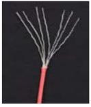
Each cord is made up of seven two-ply yarn cores braided inside a braided 100% nylon sheath giving it a relatively smooth outer texture while supplying excellent strength and durability
